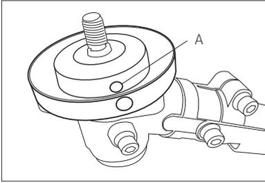
Rotate the gear box shaft until the hole in the holder A lines up with the slot in the metal guard.
