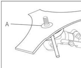
Place the 3 tooth blade on the holder A, centring the blade on the raised centre.
