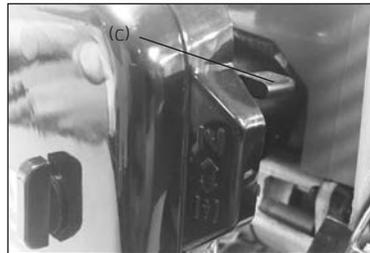
Fig 2 - Move the choke lever (c) to the closed (
