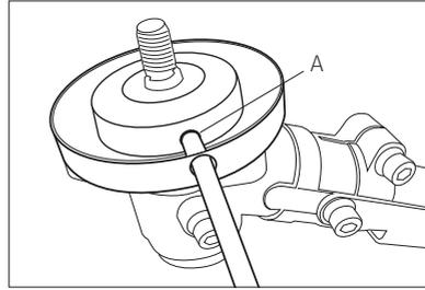
Insert an Allen key or screwdriver into the hole in the gearbox cover and into holder A.
