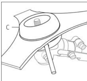
Fit the domed nut protector C over holder B and the blade.
