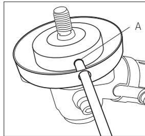
Insert an Allen key or screwdriver into the hole in the gearbox cover and into holder A.
