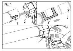
**NOTE** Fit the second tube with a flat or round end depending on the type of work to be accomplished. To remove the first tube (1), insert the screwdriver included in the kit in the hole (5) and press firmly until you can slide the tube out from the air outlet nozzle.v
