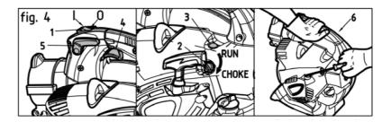
**IMPORTANT** To avoid breaking the starter rope, do not pull the whole length of it or let it slide along the edge of the rope guide hole. Release the starter gradually, to avoid letting it fly back uncontrollably.
