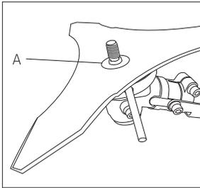
Place the 3 tooth blade on the holder A, centering the blade on the raised centre.
