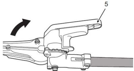
6. Release the red locking lever and ensure the locking pin (3) engages with the quadrant.
