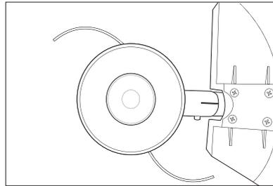
Make sure that the nylon head is securely locked in position and remove the Allen key.
