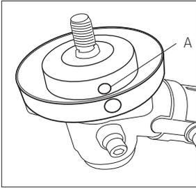
Rotate the gear box shaft until the hole in the holder A lines up with the slot in the metal guard.
