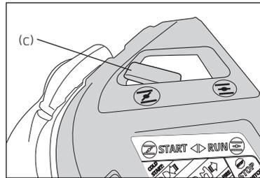
Fig 2 - Move the choke lever (c) to the START (
