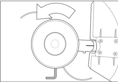
Screw the nylon head anti-clockwise (turn left) onto the threaded shaft on the end of the gearbox.
