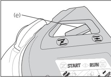
Fig 5 - Move the choke lever (e) to the RUN ( ||| ) position.
