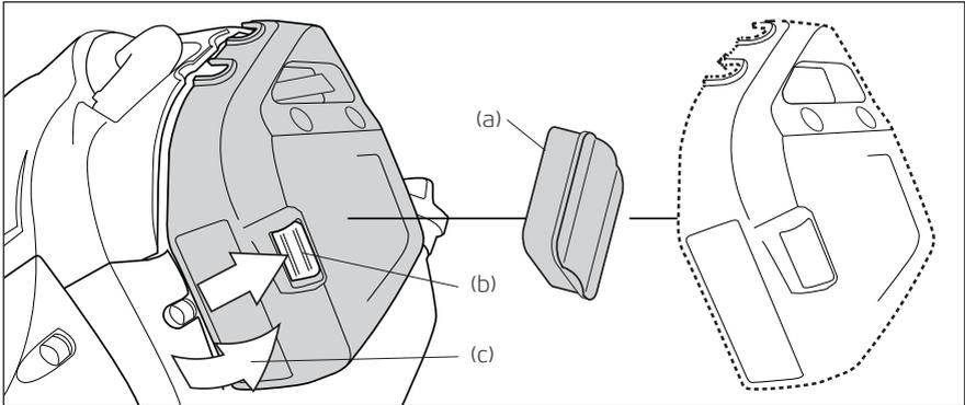
Before using the Multi-Tool, check the air filter (a). Being clogged, will reduce the engine performance. Remove the air filter cover by pressing on the filter cover release (b) and opening the filter cover (c). Clean the filter element in warm, soapy water, dry completely before installing. If the element is broken or shrunk, replace with a new one.
