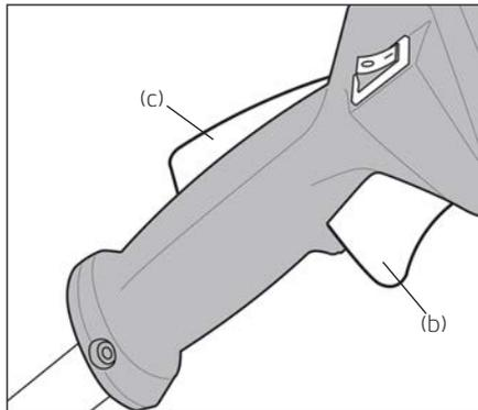
The safety lock is to prevent the throttle lever from accidentally being engaged. The throttle lever (b) can only be pressed in if the safety lock (c) is held down. Check if the safety lock and throttle levers return to their original position and the engine returns to idling when you release your hand from the handle.
