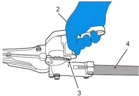
5. While holding the shaft (4), move the cutting head to the desired position.
