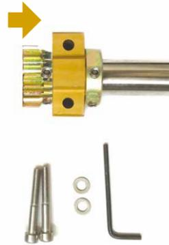
Slide the following parts onto the Control Tube on the left hand end in the following order, loosening the Grub Screws before sliding each item on.
