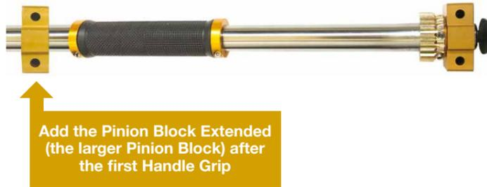
**Add the Pinion Block Extended (the larger Pinion Block) after the first Handle Grip**
