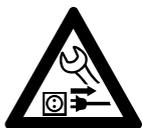
Before starting any work on the machine: Always disconnect the machine from the mains power supply.
