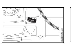
Before fueling, clean the filler cap and the area around it to ensure that no dirt falls into the tank.
