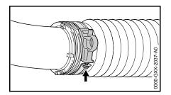
• Tighten down the screw (arrow).
