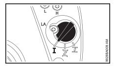
Choke knob automatically returns to the run position I when the throttle trigger is operated.
