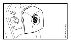
Turn the filter cover lock (1) counterclockwise to the vertical position.
