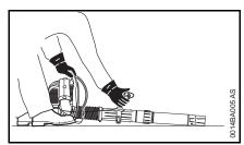
Place the unit securely on the ground and make sure that bystanders and loose objects are well clear of the nozzle outlet.  Make sure you have a firm footing: Hold the unit with your left hand on the carrying handle and grip the control handle with your right hand.
