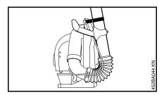
Secure the blower tube to the handle on the backplate with the hook and loop fastener.
