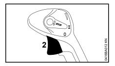
Operate the throttle trigger (2).
