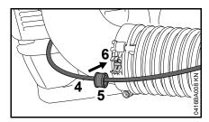
• Engage the throttle cable (4) with sleeve (5) in the hose clamp (6).
