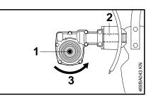
The axle (1) must be below the shaft (2). Direction of rotation (3) of MultiTool.
