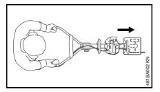
Operate the MultiEngine with FC-MM edger in the forward direction only.
