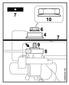
• Position the blade (7) on the thrust plate (8).
