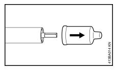
Pull the protective caps off of the ends of the shaft and keep them in a safe place for later use – see "Storing the Machine"
