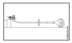
Place the edger so that the blade mounting (1) faces upwards
