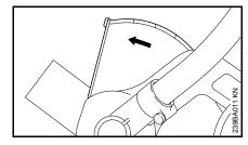
The arrow on the deflector shows the direction of rotation of the blade – see "Use".
