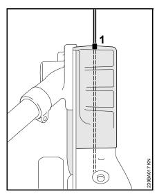
Use the gunning sight (1) for the cutting blade to align the blade to the edge
