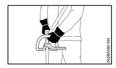
On models with a loop handle and barrier bar, left hand on loop handle, right hand on control handle, even if you are left-handed.
