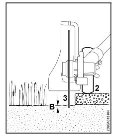
The depth of cut is influenced by uneven ground as well as height and working position of the operator. For this reason,
