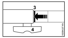
When correctly installed, the red line (3) (arrow point) must be flush with the end of the coupling sleeve.
