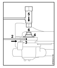
Insert the stop pin (2) into the hole (3) as far as stop – apply slight pressure and turn back and forth together with the thrust plate (4) until the pin slips into position and blocks the shaft.
