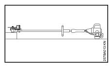
Lay the power edger on its back so that the blade mounting (1) faces up.
