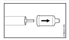
Pull the protective caps off the ends of the drive tube and keep them in a safe place for later use – see "Storing the Machine".
