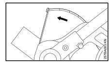
The arrow on the deflector shows the direction of rotation of the blade – see "Using the Unit".
