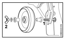
End of screw thread (1) is deformed so that the wingnut (2) cannot be lost
