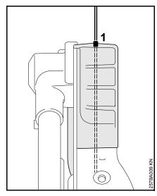
Use the gunning sight (1) to line the blade up with the edge of the bed.
