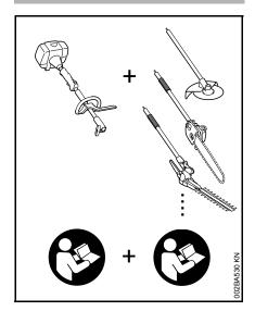
In the STIHL KombiSystem a number of different KombiEngines and KombiTools can be combined to produce a power tool. In this instruction manual the functional unit formed by the KombiEngine and KombiTool is referred to as the power tool.
