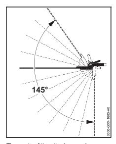
The angle of th cutter bar can be adjusted upwards in 4 stages from 0° (straight) to 55°, and downwards in 7 stages from 0° to 90° (right angle facing down). There are therefore 12 possible working positions.
