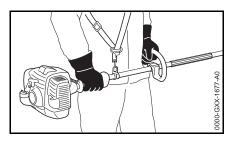
Right hand on control handle, left hand on loop handle on drive tube, even if you are left-handed. Wrap fingers and thumbs firmly around the handles.
