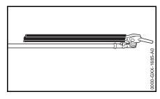
The cutter bar can be folded flat against the drive tube and locked in position to save space during transportation.
