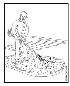
Working position and method are the same as for a brushcutter: Sweep the cutter bar to and fro in an arc just above the ground.
