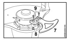
Place the bumper (7) on the pegs (8) and locators in the deflector and secure in position with the two screws (9).
