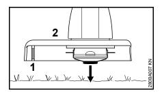
Hold the rotating mowing head above the ground – tap it on the ground once – about 3 cm fresh line is advanced.
