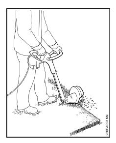
The unit can be quickly converted into a power edger (see "Converting Unit to Power Edger").
