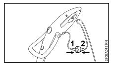
Insert the plug (1) into the extension cord coupling (2).
