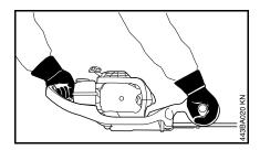
Left hand on the control handle, right handle on the front handle. Wrap fingers and thumbs firmly around the handles.
