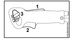
The slide control (3) is in the normal run position  ${\bf I}$ .
