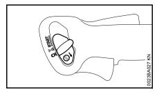
Move the stop switch in the direction of 0 – when released, the slide control springs back to the normal run position I.
