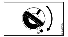
While holding the cap depressed, turn it clockwise until it engages in position.
