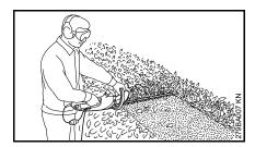
If the hedge is wide, cut it in several passes – one hand on the front switch lever – one hand on the control handle.
