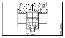
Guide the PowerSweep at right angles to the direction of travel (1). Sweepings are thrown forwards, ahead of the operator.
