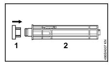
Push the grass shield (1) onto the axle (2) as far as stop.
