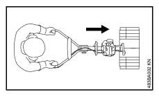
The MultiEngine with sweeping attachment is operated in the forward direction only.
