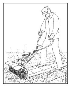
The KB-MM bristle brush MultiTool is used for cleaning areas and paths, including uneven and jointed surfaces, and natural stone paving.
