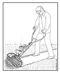
The KW-MM PowerSweep MultiTool is used for sweeping areas and paths, moving wet materials, such a leaves or dirt to a central point, clearing snow and removing standing water from solid surfaces.
