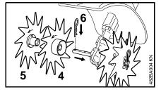
Rotate the inner right-hand blade (4) on the axle until it can be pushed into position – check the direction of rotation again (arrows).
