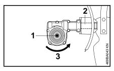
The axle (1) must be below the shaft (2). Direction of rotation (3) of MultiTool.
