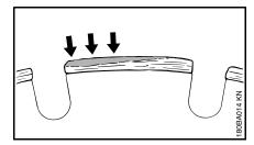
Built-up edges take the form of a light gray deposit on the tops of the diamond segments. This deposit on the segments clogs the diamonds and blunts the segments.
