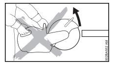
Whenever possible, do not use the upper quarter of the abrasive wheel for cutting. Use extreme caution when entering the abrasive wheel in a cut, do not twist or push into the cut
