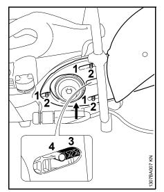
Press the oblong holes (1) in the "cast arm and guard" on to the studs (2), guiding the ribbed V-belt over the front pulley
