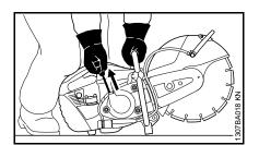
Place the cut-off machine carefully on the ground, ensuring that the abrasive wheel cannot touch the ground or any objects. There must not be anyone within the swivel range of the cut-off machine
