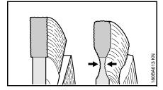
Do not cut into the base course (frequently chipped stones and gravel) when cutting roadway pavement – cutting in chipped stones and gravel is revealed by light-colored dust – excessive undercut may occur as a result – **Danger of shattering!**
