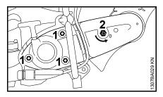
Prior to tensioning of the ribbed V-belt, the nuts (1) must be loosened and the arrow on the tensioning nut (2) must point to  $\mathbf{0}$ .
