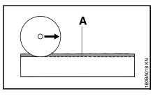
• Grind a guide groove (A) along the line marked
