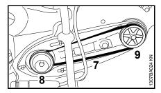
Carefully insert the new V-belt (7) on the V-belt pulley (8) on the engine and the front V-belt pulley (9)
