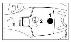
Unscrew screw (1) and remove cap (2) – screw (1) is secured in the cap (2) to prevent loss
