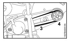
• Remove the V-belt (3) from the front pulley (4)
