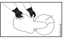
Always hold the machine **firmly with both hands**: Right hand on the rear handle – even if you are left-handed. To ensure reliable control, wrap your thumbs tightly around the handlebar and handle.
