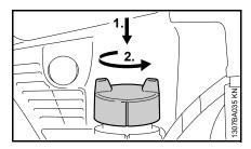
Press the filler cap down as far as possible by hand, then turn it counterclockwise (approx. 1/8 turn) and remove
