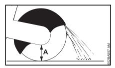
The procedure is dependent on the outer diameter of the pipe and the maximum possible cutting depth of the abrasive wheel (A).
