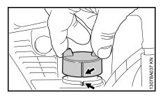
Grip the cap – the cap is closed properly if it cannot be removed and the markings (arrows) on the cap and fuel tank are aligned If the cap can be removed or the markings do not align, close the cap again – see sections "Closing the filler cap" and "Checking the lock".
