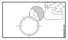
• First lateral cut on the top half of the pipe
