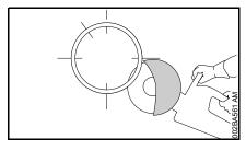
• Use the upper quarter of the abrasive wheel for cutting the opposite lower side.
