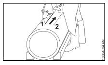
• Always make severing cuts so that the abrasive wheel is not pinched
