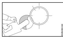
Always start at the bottom, use the upper quarter of the abrasive wheel for cutting
