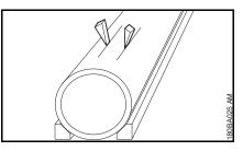
Use wedges and/or leave ridges that are broken after cutting
