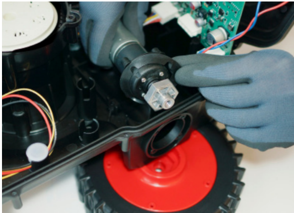
Remove wheel motor and gasket.
