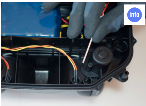
When mounting, be sure to press in the loop sensors with a soft pin (such as wood).
