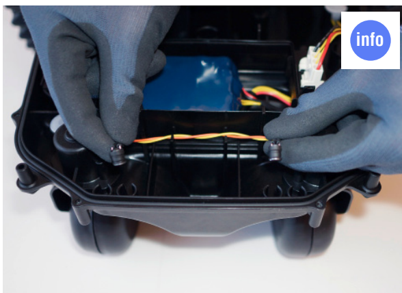
Gently release sensors in upward direction. When assembling pay attention to color coding.
