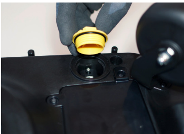
Unscrew USB protection cap.
