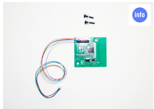
Radio board Installation note: Always use insulating washers.
