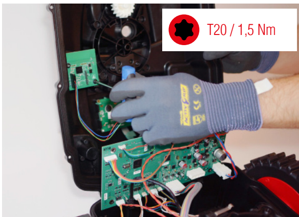
Loosen 2x screws and remove the board.
