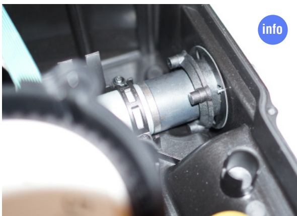
Installation note: During assembly, align sealing ring and screw guide.
