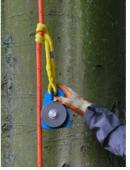
(3)Attach the RC-3100 to the prusik loop by hooking the device onto the loop by means of the prusik retention
