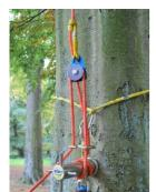
**Routing The Working Line** RC-1000 & RC-2000 Lowering Device
