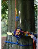
Raise the prusik loop and pulley up the line then release the working line from the fairleads leaving one wrap around the bollard
