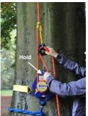
To get extra tension securely hold the end of the working line which enters the pulley. then release the line from the pulley.
