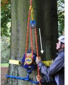
By pulling down vertically on the line exiting the pulley this will start to remove slack from the main line.
