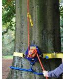
Tie off the working line and repeat the process over until the desired tension has been achieved
