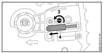
Turn the tensioning screw (3) counterclockwise until the tensioner slide (4) butts against the left end of the housing.
