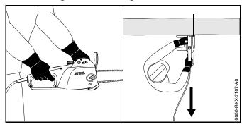
Hold and control your saw with your left hand on the front handle and your right hand on the control handle. Wrap thumb of left hand around the front handle and thumb of right handle around the control handle.
