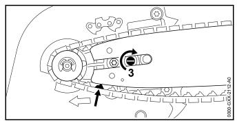
Turn the tensioning screw (3) clockwise until the chain fits snugly against the bar. Make sure the drive link tangs engage the bar groove.
