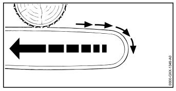
The saw is pushed back toward the operator when the top of the bar is used for cutting.
