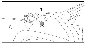
Depress the reset button (1). The reset button (1) engages in position. The circuit is no longer interrupted.
