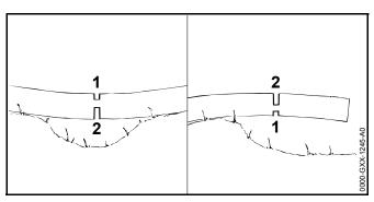
► If the limb is under tension: Make the relieving cut (1) at the compression side and then perform bucking cut (2) from the tension side.
