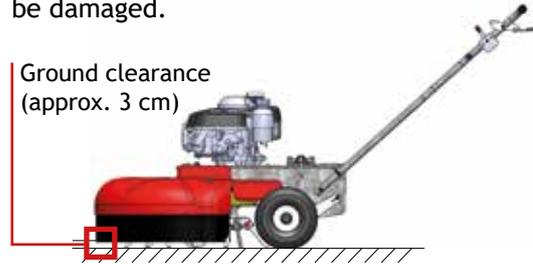
(Fig.: Ground clearance 3 cm)
